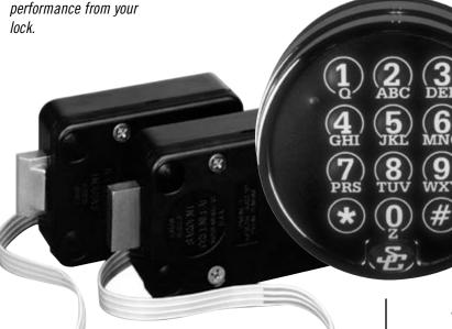
The keypad base diameter is 4" (101,6 mm). This is slightly greater than the diameter of standard S&G dial rings for mechanical locks. The 6120 series keypad will cover any scratches or paint blemishes left by the old lock.
