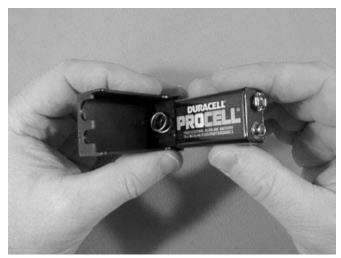
**Step 3**—Note that the battery is oriented so that the larger contact is in line with the larger opening in the top of the battery holder. It's important to orient the new battery this way.
