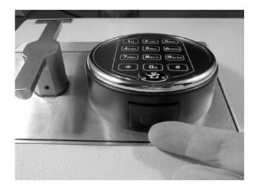
**Step 2**—As you remove the old battery, you will notice there is a spring at the bottom of the holder. The new battery will rest on top of this spring to maintain good electrical contact.
